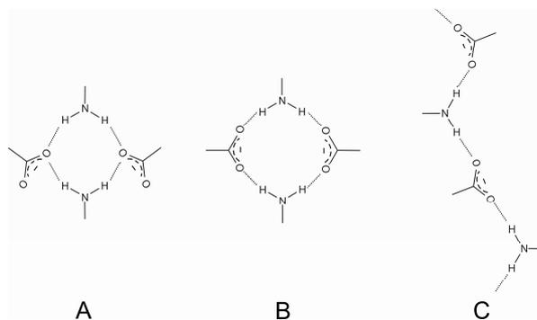
**Fig. 3.** Three types of most common synthons observed between amines/amino group and carboxylate group.
