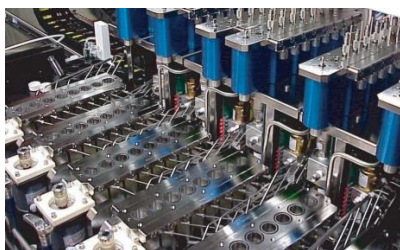
Fig. 1. Freeslate Parallel Pressure Reactors PPR48 used in olefins (co)polymerization process.
