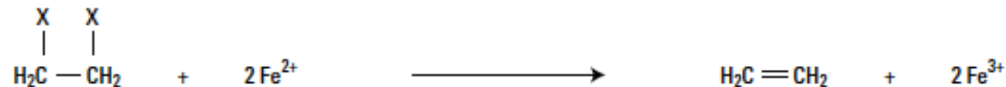
Figure 3.31. Example of a reductive transformation: electron transfer from \text{Fe}^{2+} to 1,2-dihalogen substituted ethane (X denotes a halogen atom).
